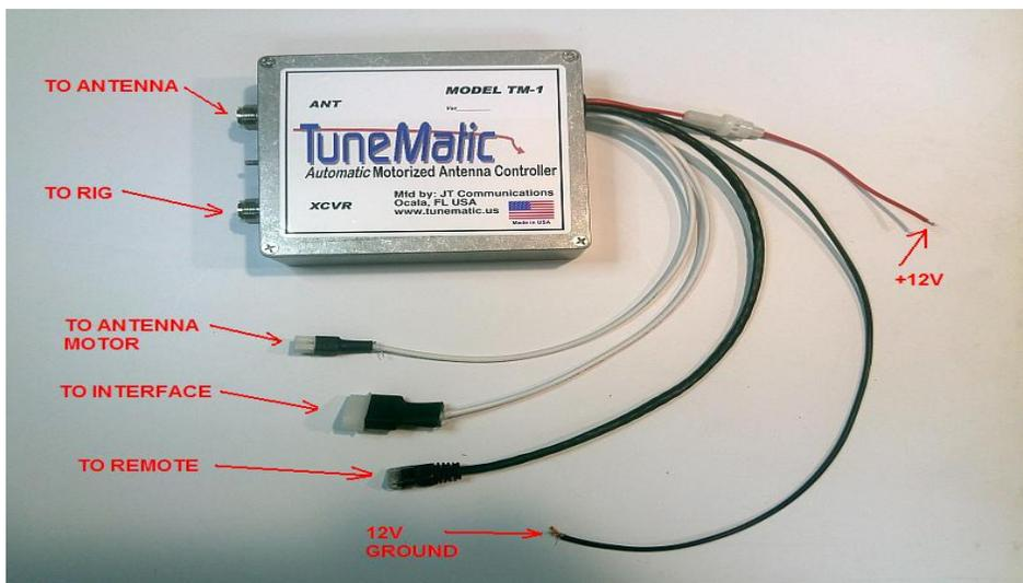
1) 12v power leads: These leads can be paralleled with radio power if desired, as they draw no current until TuneMatic is powered up by Radio Control cable. **NEGATIVE GROUND SYSTEM ONLY!**
