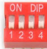
\*Most of the larger antennas can be set to 900 or 1100 mA, depending on operating temperature. **NOTE: IT IS IMPORTANT TO SET THIS LIMIT PROPERLY, as damage can occur to the antenna motor if set too high, or will prematurely trip if setting is too low.**
