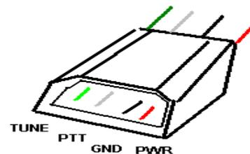
GND (BLACK [pin 2]) connects to radio ground or common.
